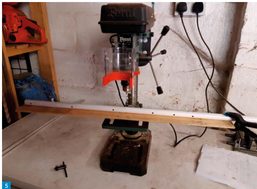
Fig. 1: Drilling the tubing to take the extension.
