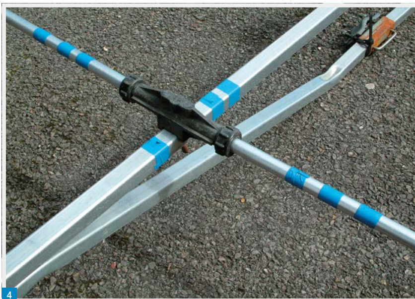
Fig. 4: Tape used to identify the elements on the boom of a 6m Yagi.
